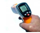
This infrared thermometer is used for measuring the temperature of the object'sSurface.Temperature range-50°C to +420°CAccuracy±1.5°c or ±1.5%Resolution0.1°C or 0.1°FDistance to Spot Size12 : 1
