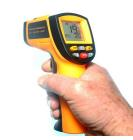
This infrared thermometer is used for measuring the temperature of the object'ssurface.Temperature range $-50^{\circ}$ C to  $+700^{\circ}$ CAccuracy $0-700^{\circ}$ C  $\pm 1.5\%$  or  $\pm 1.5^{\circ}$ C,  $-50-0^{\circ}$ C  $\pm 3^{\circ}$ CResolution $0.1^{\circ}$ C or  $0.1^{\circ}$ F
