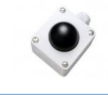
A radiation sensor measures the thermal radiation in the range of -30 up to +75°C .Range-30 to +75°CSensorPt100Protection TypeIP65Measurement Currentapprox. 1 mAHousingpolyamide with snap closing screws, colour white RAL9010
