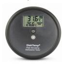
The DishTemp® dishwasher thermometer simulates a plate as it's cleaned and sanitised in a commercial dishwasher, accurately recording the maximum surface temperature at the touch of a single button. 0 to 90°C Range 0.1°C /°F Resolution ±0.5°C Accuracy **IP** Rating **IP66**
