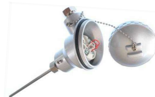
C Platinum Resistance Pt100 3 wire class B Resistance Thermometer with KNE Head and Fitted
