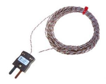
B Type T PFA Exposed Junction with Miniature Plug
