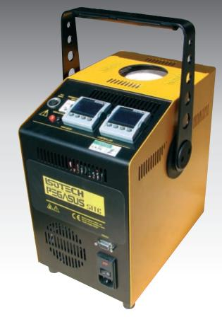
The S model has universal sensor input allowing Platinum Resistance Thermometers, Thermocouples (Types K, N, R, S, L, B, PL2, T, J and E) along with Linear Process Inputs including 4-20mA current transmitters to be displayed on the inbuilt indicator. The indicator can be programmed with up to five calibration points to provide high accuracy digital probe matching. The indicator and controller are both addressable over the communications link.
