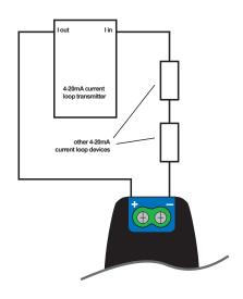
Connecting to a current loop transmitter.
