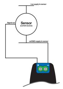
Connecting to a current source sensor.
