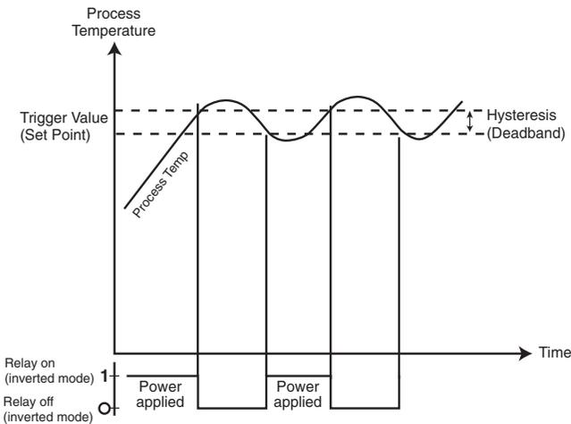
Configuration: High mode/Trigger Value = Set Point/Hystersis value 1 or 2°C\*/Polarity inverted/Use NO contact.
