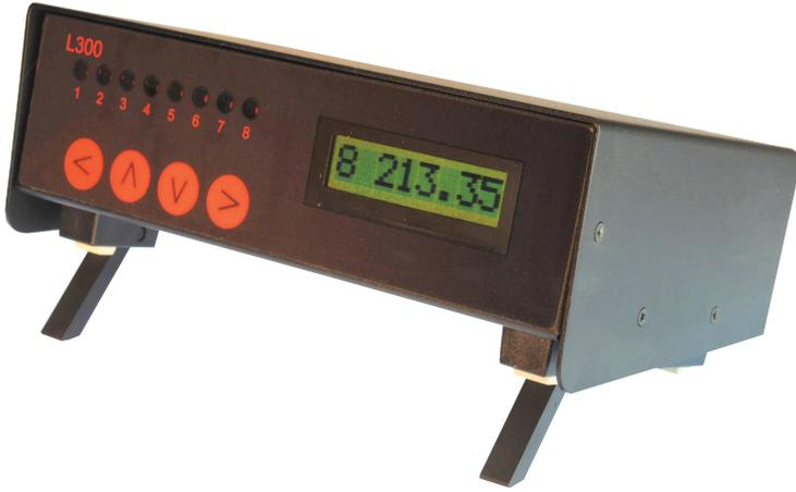
The L300 Pt100 and Thermocouple temperature alarm/ on-off controller can be used in conjunction with a PC to provide accurate monitoring and alarm or on-off control of up to 8 zones simultaneously. It can also be used as a stand-alone instrument without the need for a PC.
