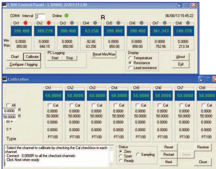
Clear the existing calibration data by clicking ‘Reset’ for the selected channel in the calibration window.
