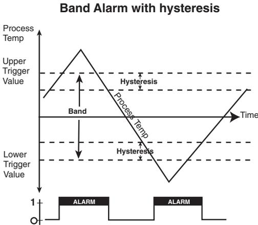
**Hysteresis** is adjustable to suit the application or the user’s requirements; the hysteresis defines a dead band within which relay switching will not occur. This is used to prevent excessive relay cycling which could compromise relay contact reliability and process stability. The alarm mode diagrams illustrate how hysteresis works (refer to the relay on/off states below each diagram for clarity).
