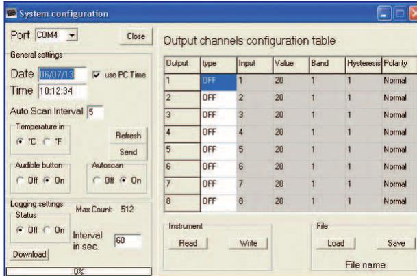
In this window, the Comms Port is selected and instrument settings are made.
