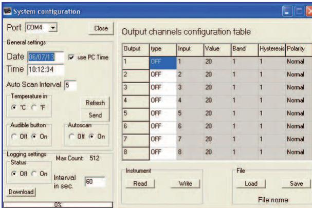
The logging interval for each channel is set up (common) and sent to the instrument by clicking 'send'.
