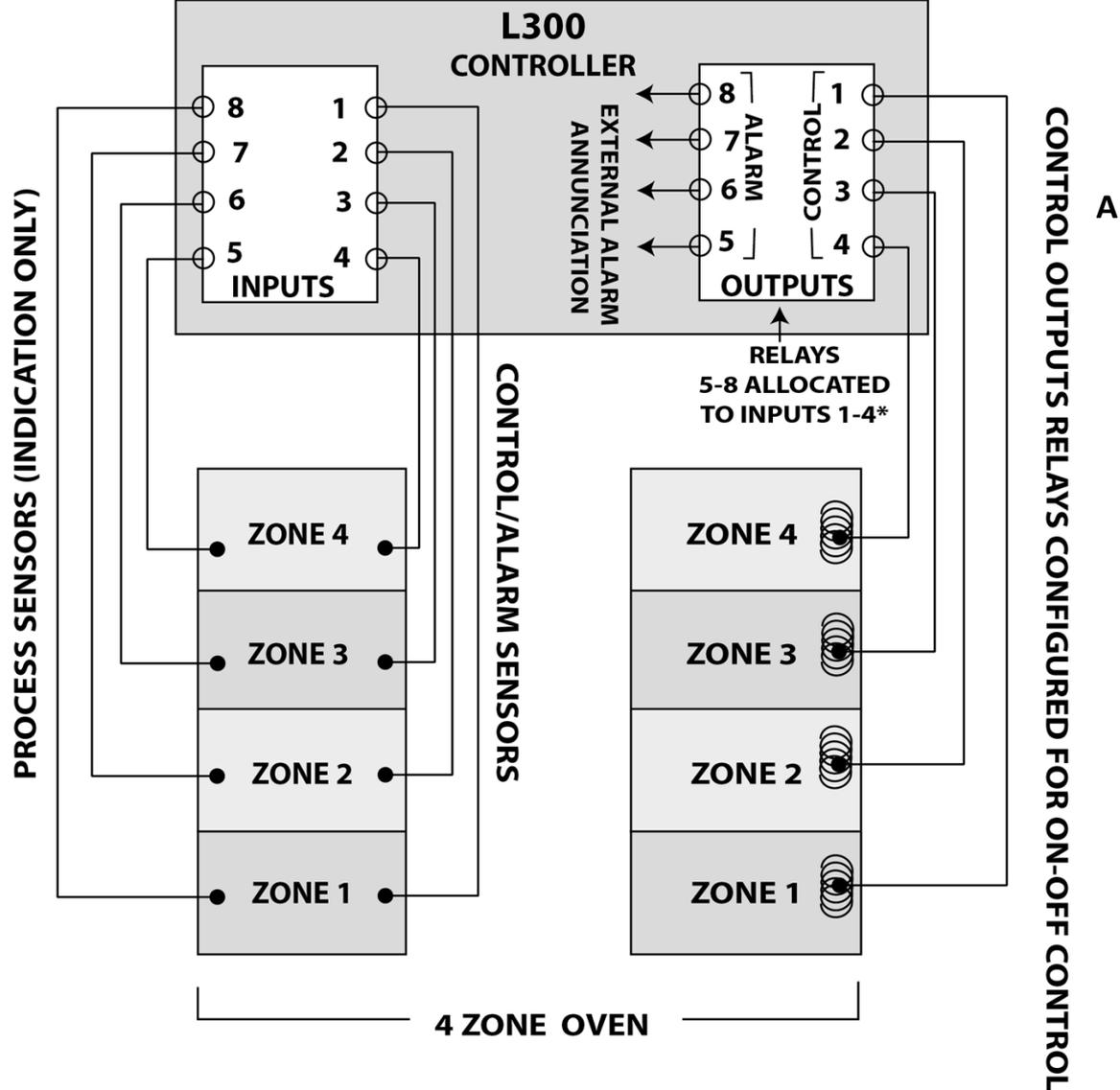
\*ALARM OUTPUTS STATUS IS INDICATED BY L300 FRONT PANEL LEDs
