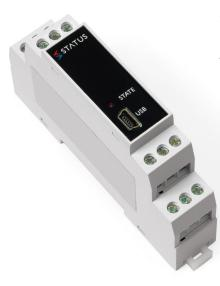
**BASIC FREQUENCY MODE** - Input frequency range is taken, any values within the maximum (0 to 65) KHz can be used, and converted to an analogue output. The analogue output can be (0 to 20) mA, (4 to 20) mA, (0 to 10) V, (-10 to 10) V or any part of the output range that is required.
