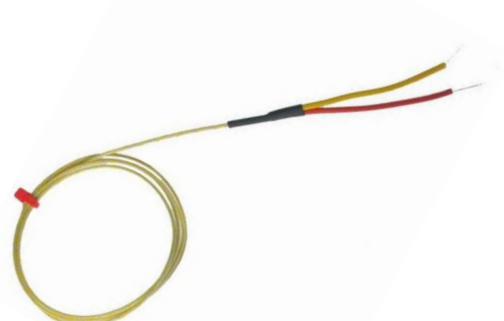
B Glassfibre insulated Exposed Junction Thermocouple with Bare Tails
