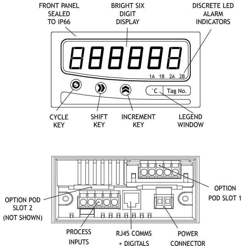
The diagram below shows the rear panel positions for all electrical connections.
