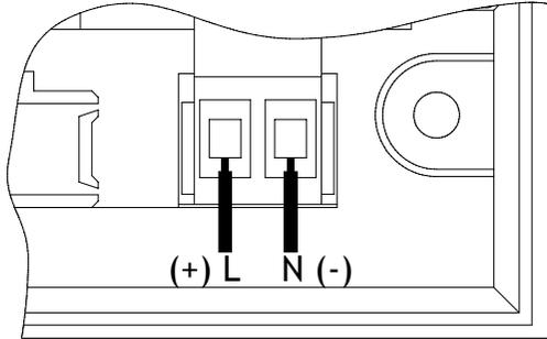
Wires are retained by screws. Ensure that the exposed section of the wire is fully inserted and that no loose strands are exposed.
