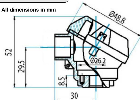
This unit is available with two styles of probe entry, M10 x 1.0 or 1/8" BSP. The unit must be installed with adequate protection from moisture and corrosive atmospheres. The cable entry is M16, the correct type cable gland must be used to match cable size and operating environment and provide protection to at least IP54. Care must be taken with device location to ensure the ambient temperature does not exceed the specified operating temperature.
