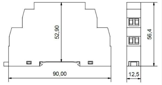
The equipment must be mounted on a DIN rail style DIN EN50022 inside a plastic or metal enclosure with a protection level  $\geq$  IP65. All wiring must be secured. Maximum cable sizes 2.5 mm<sup>2</sup>. Connection is via screw clamp terminals.
