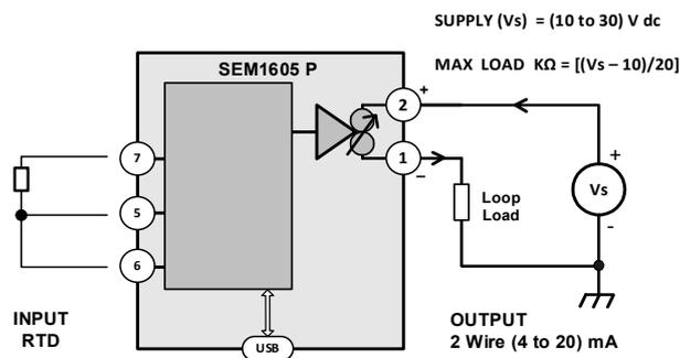
It is good practice to ensure that the (4 to 20) mA loop is grounded at a single point in the loop.
