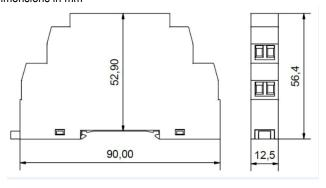
The equipment must be mounted on a DIN rail style DIN EN50022 inside a plastic or metal enclosure with a protection level >= IP65. All wiring must be secured. Maximum cable sizes 2.5 mm<sup>2</sup>. Connection is via screw clamp terminals.
