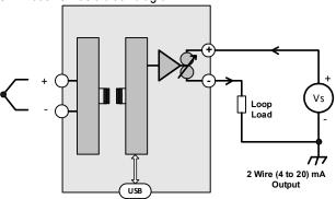
It is good practice to ensure that the (4 to 20) mA loop is grounded at a single point in the loop.
