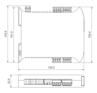
The equipment must be mounted on a DIN rail style DIN EN50022 inside a plastic or metal enclosure with a protection level >= IP65. All wiring must be secured. Maximum cable sizes 2.5 mm. Connection two-part screw terminals.
