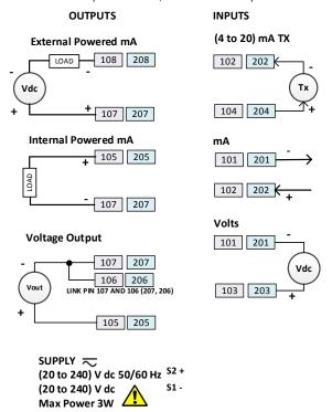
Input connections for cable length >3 metres: use screen or twisted pair cables. Max cable run 30 metres.
