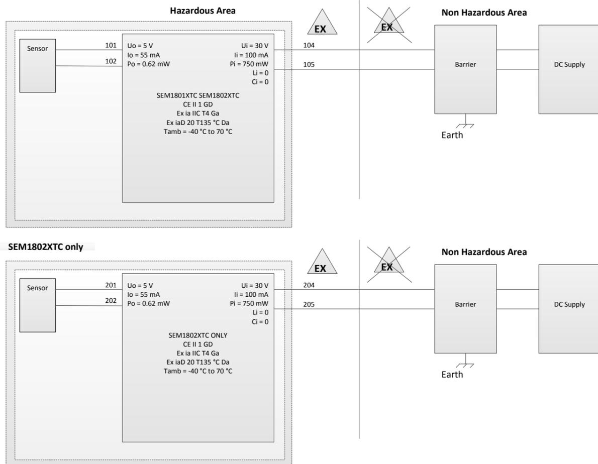
Sensor wires must be isolated from earth breakdown voltage 500 V dc
