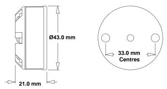
Mounting holes: two holes 5.5 mm diameter, 33 mm centres. Centre hole sensor wire entry 4 mm.
