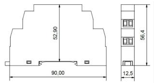
The equipment must be mounted on a DIN rail style DIN EN50022 inside a plastic or metal enclosure with a protection level >= IP65. All wiring must be secured. Maximum cable sizes 2.5 mm<sup>2</sup>. Connection clamp terminals.
