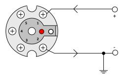
Use twisted pair or screened cables for cable lengths greater than 30 metres. Maximum cable length 1000 metres.
