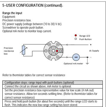
Set the precision resistance box representative value for high scale (20 mA out) sensor resistance.
