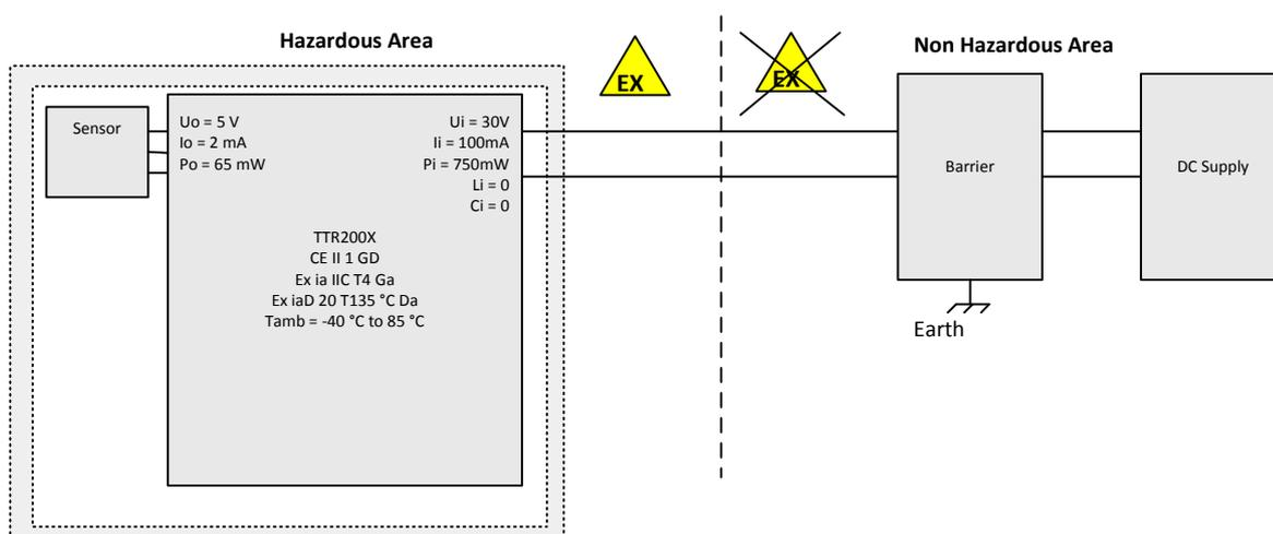
Sensor wires must be isolated from earth breakdown voltage 500 V dc
