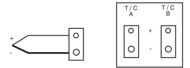
Thermocouple(s) must be fitted with an appropriate compensating standard plug and connected to input T/C A and/or T/C B as required. When using an external cold junction (e.g. ice referencing), copper-copper (not compensating) plugs should be used.
