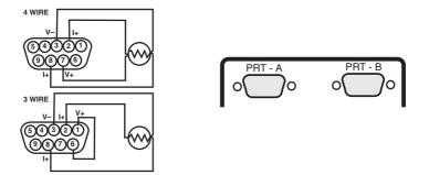
Platinum resistance thermometers must be fitted with a high quality D-plug and connected to input PRT-A and/or PRT-B as required. A 3 or 4 wire configuration can be used but they are connected differently as shown. The instrument will automatically sense which configuration is employed.
