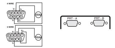
Platinum resistance thermometers must be fitted with a high quality D-plug and connected to input PRT-A and/or PRT-B as required. A 3 or 4 wire configuration can be used but they are connected differently as shown. The instrument will automatically sense which configuration is employed.
